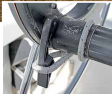
The autopilot clutch lever which I have found, like others before me, disengages by itself
